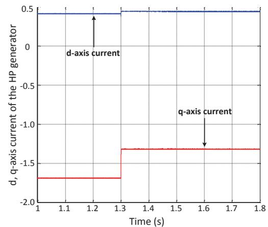
Fig. 11. The d, q-axis current characteristics of the HP generator in the proposed AC/DC hybrid generation system
