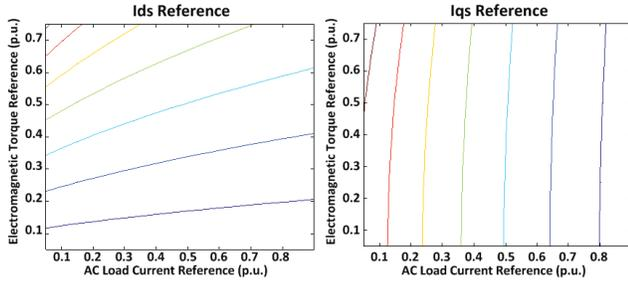
Fig. 6. Contour maps of d-q axis current commands for AC load current and generator torque reference sweep test
