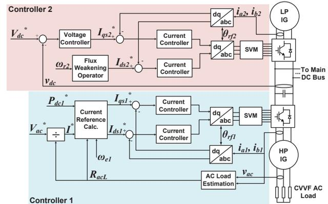
Fig. 7. Closed-loop control scheme for the proposed AC/DC hybrid generation system
