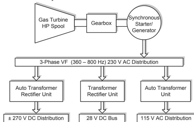
Fig. 1. System configuration of the synchronous generator based AC primary generation system
