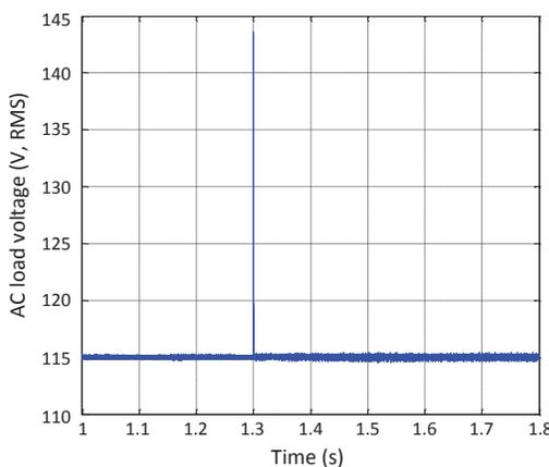
Fig. 9. The AC load voltage regulation characteristics of the proposed AC/DC hybrid generation system
