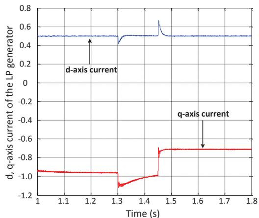
Fig. 12. The d, q-axis current characteristics of the LP generator in the proposed AC/DC hybrid generation system
