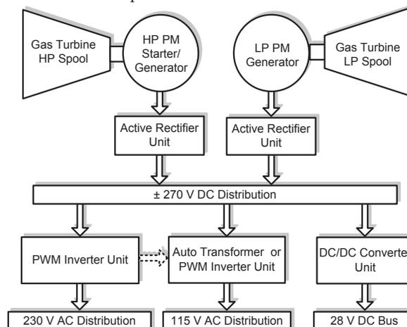
Fig. 2. System configuration of the permanent magnet generator based DC primary generation system
