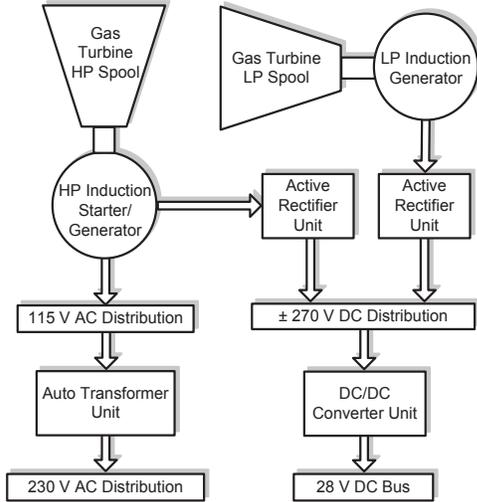
Fig. 3. System configuration of the induction generator based AC/DC hybrid generation system
