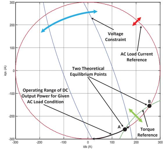
Fig. 5. Operating constraints of the high pressure spool generation subsystem
