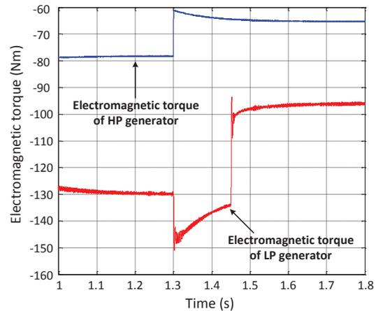
Fig. 10. The electromagnetic torque characteristics of HP and LP generators in the proposed AC/DC hybrid generation system
