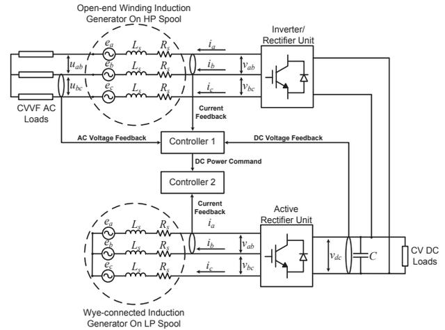
Fig. 4. Electrical system diagram of the induction generator based AC/DC hybrid generation system
