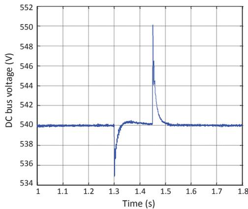
Fig. 8. The DC bus voltage regulation characteristics of the proposed AC/DC hybrid generation system
