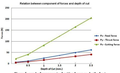
Figure 5:-graph of components of cutting forces vs. depth of cut
