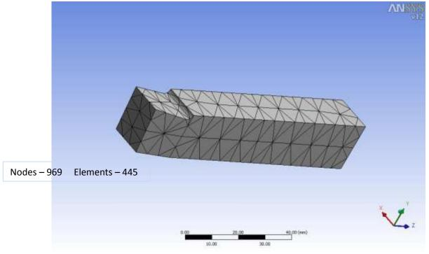
Figure 7:- mesh model made by ansys software
