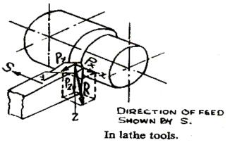
Figure 3: - components of cutting forces
