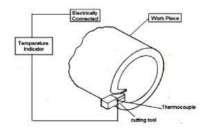
Figure 1:-Temperature Measurement in Metal Cutting
