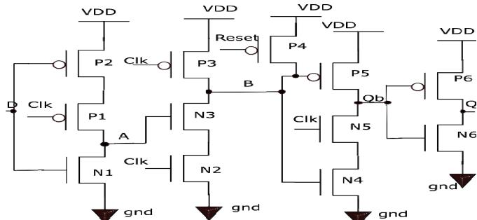
Fig. 1. Positive edge triggered TSPC DFF.
