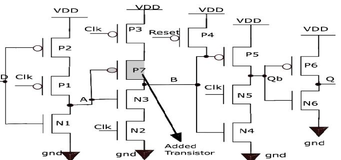
Fig. 3. Positive edge triggered MTSPC DFF.
