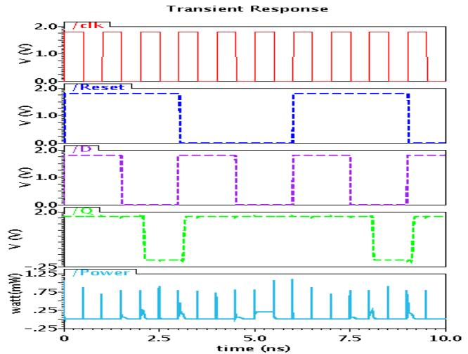
Fig. 4. Simulation results of MTSPC DFF.
