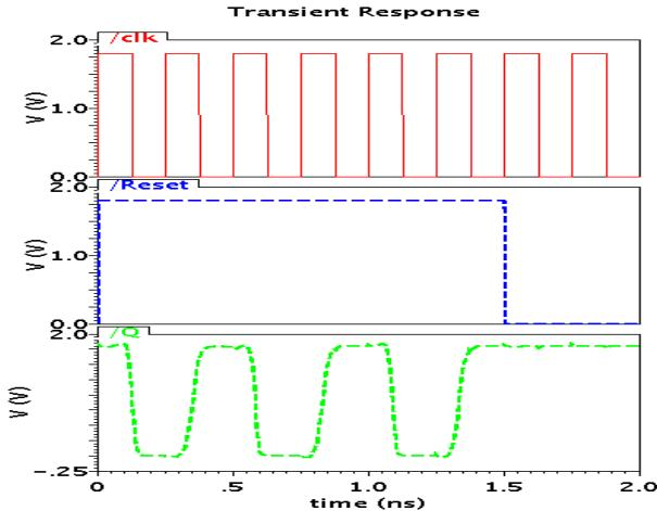
Fig. 6. Simulation results of toggle mode MTSPC DFF.
