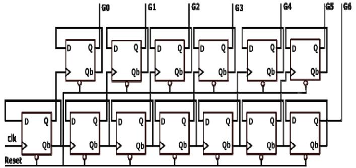
Fig. 7. 7-bit asynchronous gray code counter.
