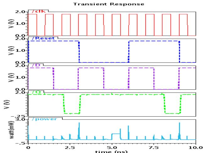
Fig. 2. Simulation results of TSPC DFF.
