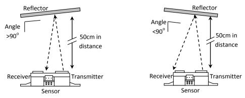
Figure 4.0: Reflector's illustration due to manual fabrication on the reflector's track in a farthest distance
