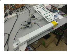
Figure 3.0: Overview of Kaptoris DAQ system and power window regulator
