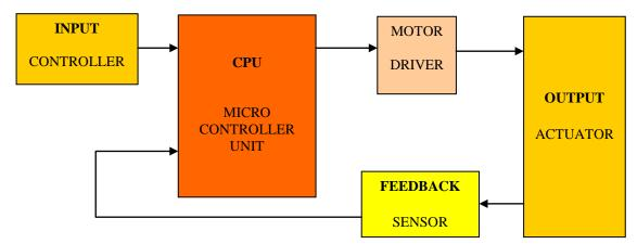
Figure 2.8: Integrated control system block diagram
