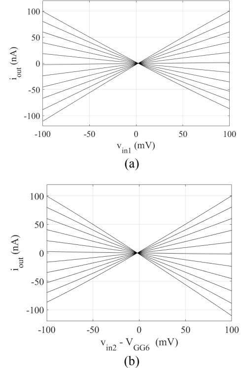
Fig. 3. Multiplier DC transfer characteristics: (a)  $i_{out}$  vs.  $v_{in1}$ , with  $v_{in2} - V_{GG6}$  varying from -100 mV to 100 mV with steps of 20 mV; (b)  $i_{out}$  vs.  $v_{in2} - V_{GG6}$ , with  $v_{in1}$  varying from -100 mV to 100 mV with steps of 20 mV. ( $V_{GG6} = 400$  mV).
