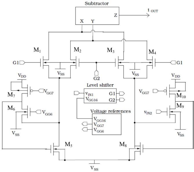
Fig. 1. Proposed CMOS analog multiplier architecture
