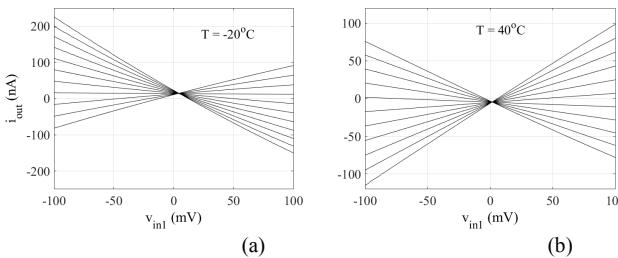
Fig. 7. Multiplier DC transfer characteristics  $i_{out}$  vs.  $v_{in1}$ , with  $v_{in2} - V_{GG6}$  varying from -100 mV to 100 mV with steps of 20 mV:
