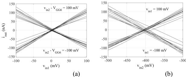
Fig. 5. Monte Carlo analysis for DC transfer characteristics: (a)  $i_{out}$  vs.  $v_{in1}$  with  $v_{in2} - V_{GG6} = \pm 100$  mV and (b)  $i_{out}$  vs.  $v_{in2}$  with  $v_{in1} = \pm 100$  mV.
