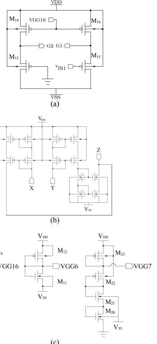
Fig. 2. Detailing of blocks in Fig.1: (a) Level shifter; (b) Current subtractor; (c) Voltage references.
