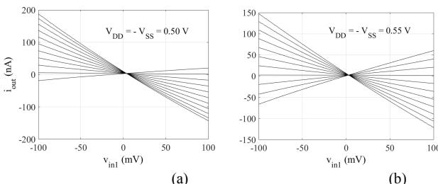
Fig. 6. Multiplier DC transfer characteristics  $i_{out}$  vs.  $v_{in1}$ , with  $v_{in2} - V_{GG6}$  varying from -100 mV to 100 mV with steps of 20 mV.
