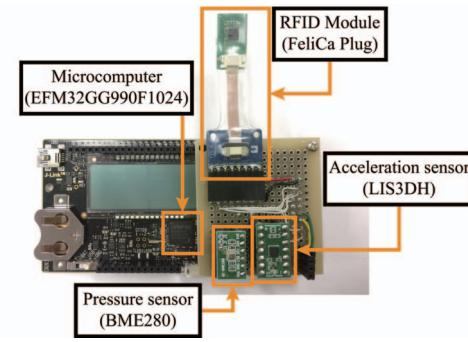
Fig. 3. Overview of developed ID card prototype.
