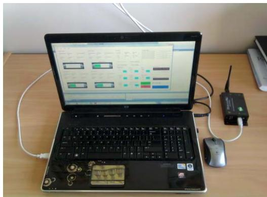
Figure 12. Central Control Station with XStream transmitter
