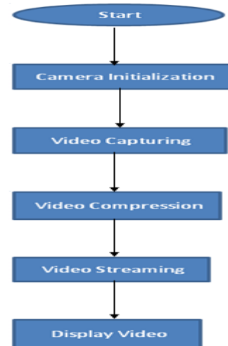
Fig. 2. Flow chart of the operation of Raspberry Pi camera
