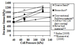
Fig 8. Variation of deviator stress at failure with cell pressure for various pavement materials
