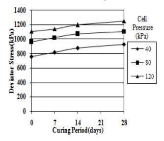
Fig 6. Variation of deviator stress at failure with curing period
