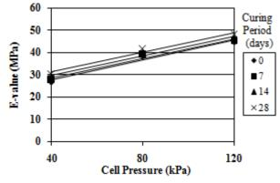
Fig 5. Variation of E-value with cell pressure
