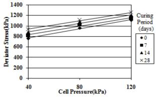
Fig 4. Variation of deviator stress at failure with cell pressure
