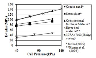
Fig 9. Variation of E-value with cell pressure for various pavement materials
