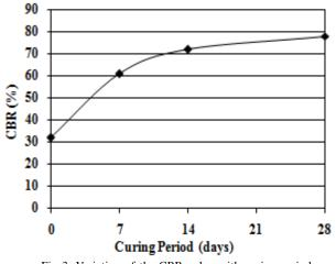
Fig 3. Variation of the CBR value with curing period
