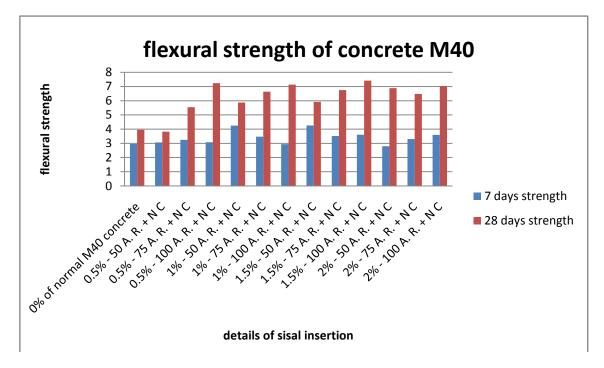
Flexural strength of concrete for M40 mix
