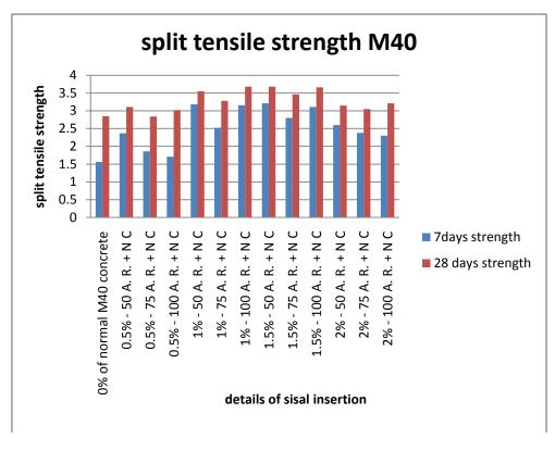
Split tensile strength of concrete for M40 mix
