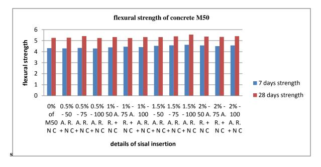
Flexural strength of concrete for M50 mix
