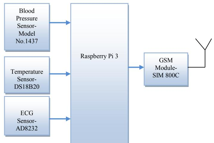
Figure 1: Client Section
