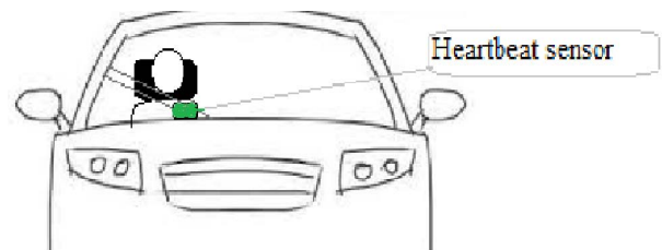
Figure 3.1 Heartbeat sensors in seatbelt
