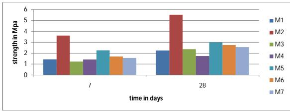
Figure 4 Flexural Tensile Strength Of Beams
