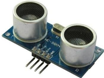
Fig 3: Ultrasonic Sensor
