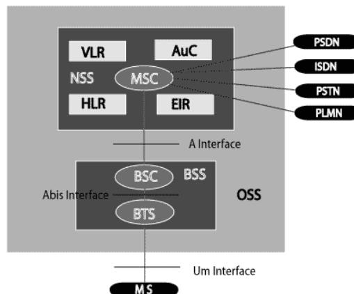
Fig 5:GSM Architecture
