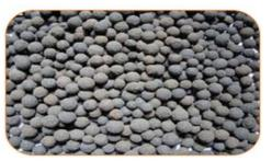
Sintered Fly ash aggregates
