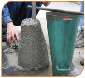
Slump cone test
