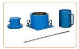
Aggregate crushing value apparatus
