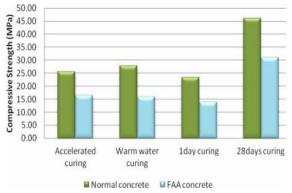
Compressive strength of normal and FAA concrete
