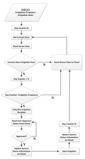
Fig. 1. Block Diagram of the Irrigation System
