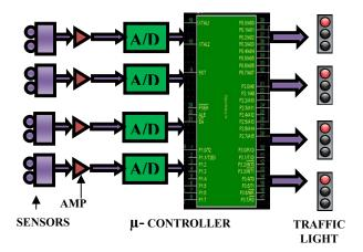
Figure. 1 Block Diagram of Intelligent Traffic Control System
