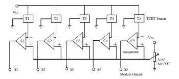
Figure. 5 Schematic Diagram of TCRT-LFSM-digital sensor [6]
