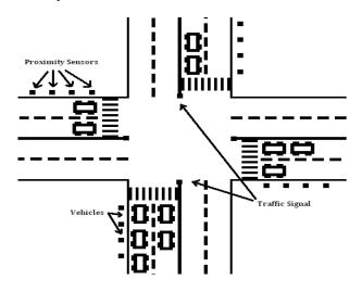
Figure. 7 Traffic System for Proposed Prototype
