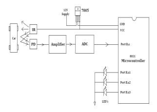
Figure. 3 Sensor Interface with Microcontroller.
