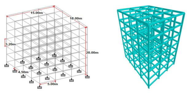
Figure 1:- Typical 3D view and Rendering View of Building
