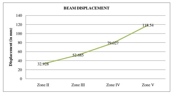
Figure 4:- Maximum Displacement in Beams
