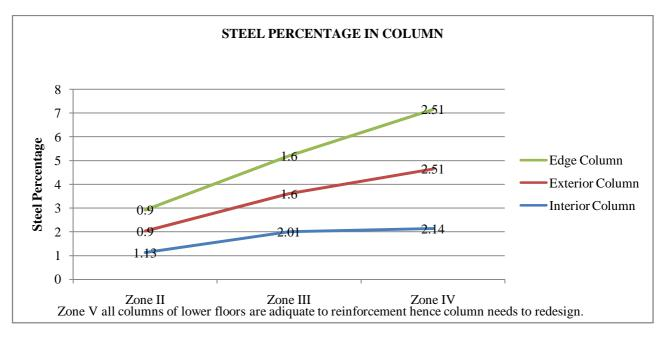
Figure 2:- Maximum Percentage of Steel in Columns
