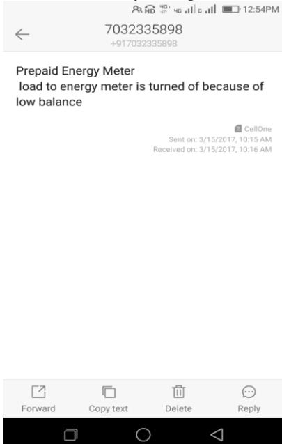
**Fig 9:** Screen shot of the SMS from GSM module for low balance
