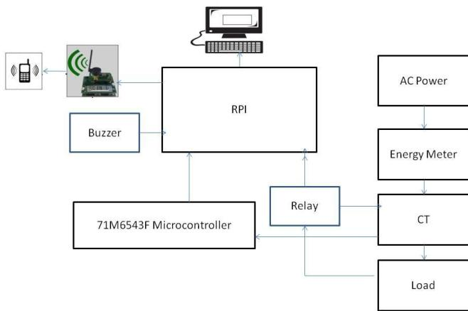
**Fig 1:** Block diagram of pre-paid electricity billing
