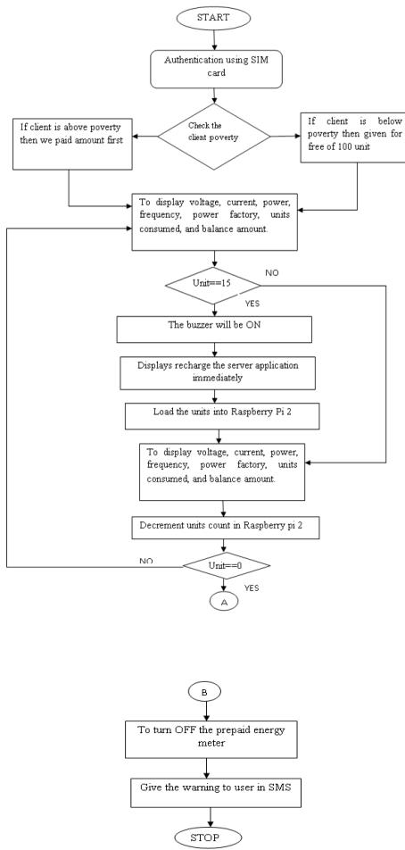
**Fig 2:** Flow chart of prepaid energy meter
