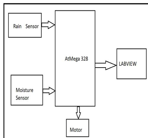
The above shown is the block diagram of the labVIEW module. soil sensor and rain sensor are used. The soil moisture sensor will read the moisture level of the soil and rain sensor will detect the rainfall. Both the data will be sent to the Arduino by sensors. Arduino is connected with the Wi-Fi module ESP8266, which will allow the wireless connection of arduino with the labVIEW software which is present on laptop. LabVIEW will then read the data received
