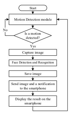
Figure 1. Flowchart for face recognition system
