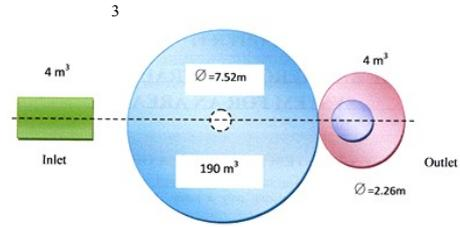
Fig. 7. Top view of digester for 15 thousand layers.
