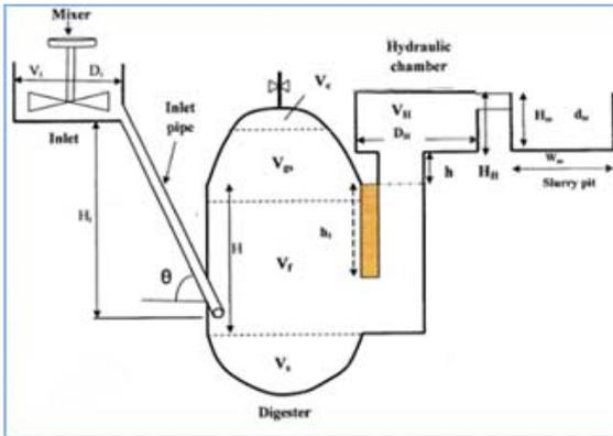
Fig. 4. Schematic diagram of biogas plant
