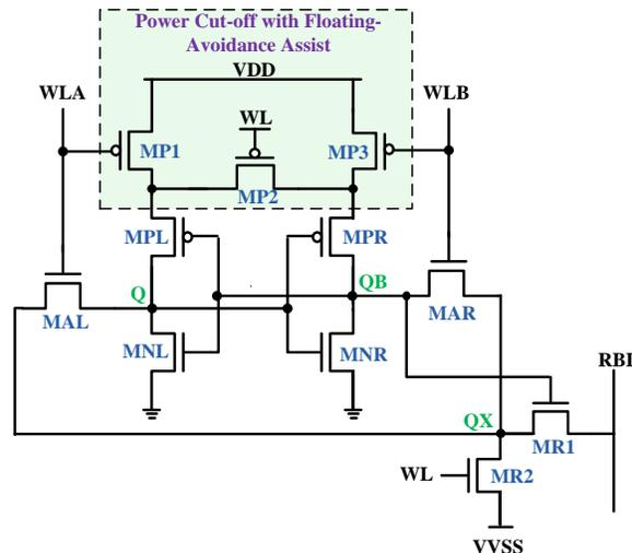
Fig. 1. Proposed 11T-1 cell schematics.
