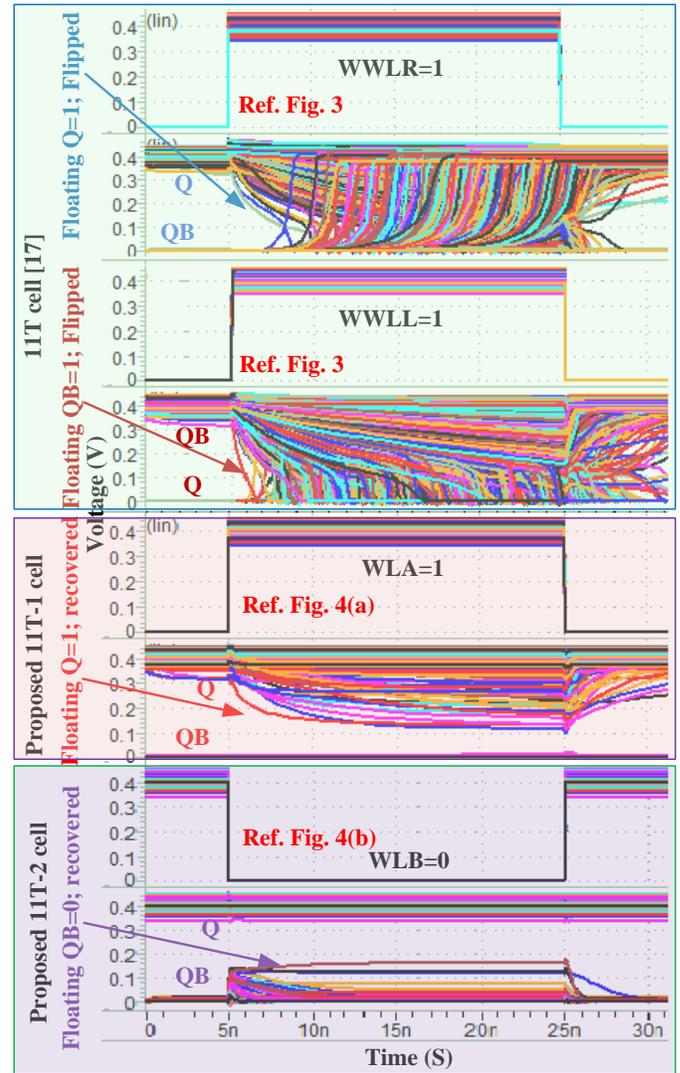
Fig. 5. Simulated transient waveform of Column Half-selected cells of various SRAM cells showing floating node conditions at TT, 25° C, and V<sub>DD</sub>=0.4V.
