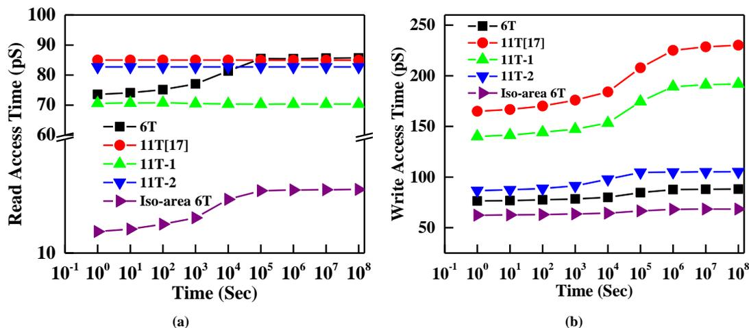
Fig. 15. (a) Read access time (b) Write access time as a function of stress time under condition of relaxed stress of 10/90.
