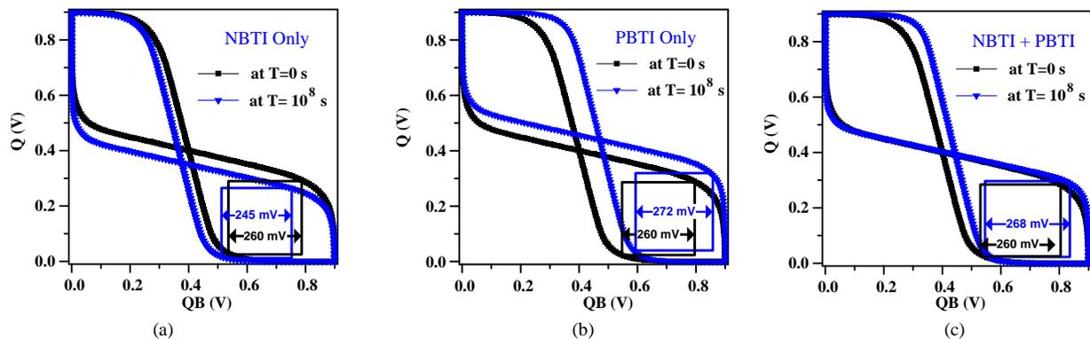
Fig. 11. Shifts in Butterfly curve to measure HSNM of 6T (RSNM/HSNM of 11T-1 or 11T-2) over the stress period of 3 years.
