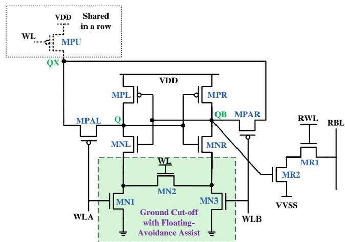
Fig. 2. Proposed 11T-2 cell schematics.
