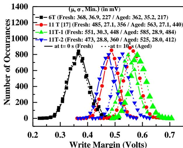
Fig. 14. Statistical distribution plot of WM for fresh and aged cell (under worst case static stress) at  $T=25^{\circ}\text{C}$  and  $V_{DD} = 0.9\text{V}$ .
