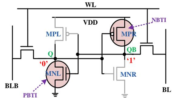
Fig. 8. 6T SRAM cell showing stress on transistors due to NBTI and PBTI.
