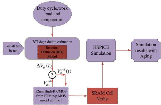
Fig. 7. Simulation flow for BTI analysis.
