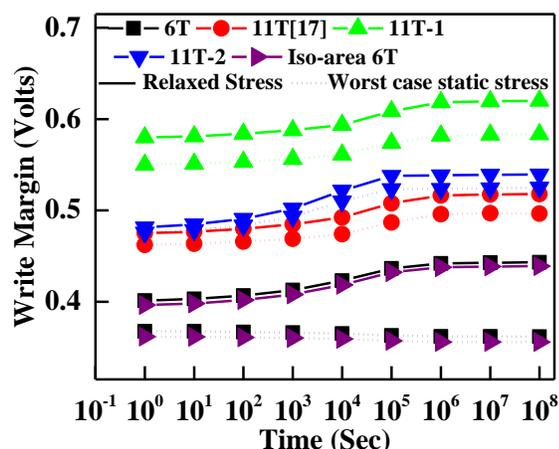
Fig. 13. Write Margin as a function of stress time under the condition of relaxed stress of 10/90.
