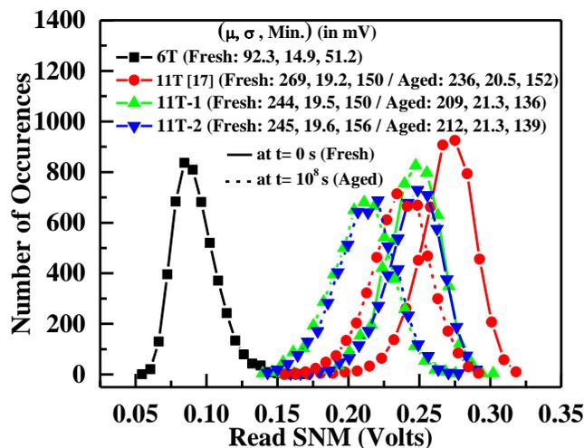
Fig. 12. Statistical distribution plot of RSNM for fresh and aged cell (under worst case static stress) at  $T=125^{\circ}\text{C}$  and  $V_{DD} = 0.9\text{V}$ . (6T suffers read failure due to high degradation at  $t=10^8\text{s}$ )
