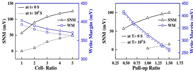
Fig. 9. SNM and WM of 6T SRAM cell as a function of CR and PR.
