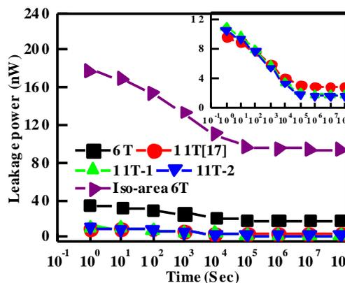
Fig. 17. Leakage power as a function of stress time under condition of relaxed stress of 10/90. (Inset: Expanded y-axis to clearly see the data)
