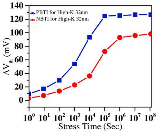
Fig. 6. Threshold voltage shift due to NBTI and PBTI for high-K and poly gate in 32nm technology node [28].
