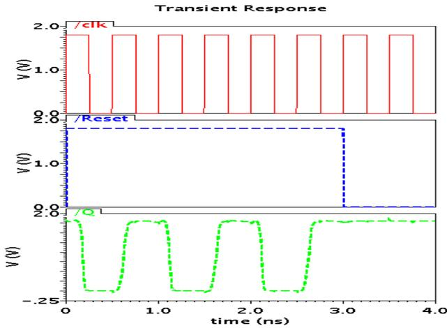
Fig. 5. Simulation results of toggle mode TSPC DFF.
