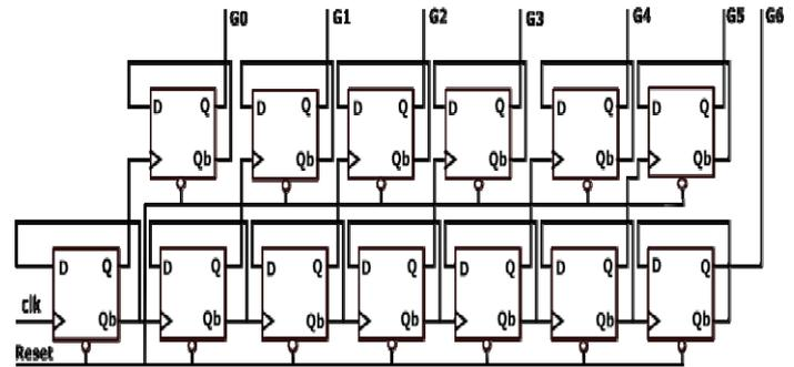
Fig. 7. 7-bit asynchronous gray code counter.
