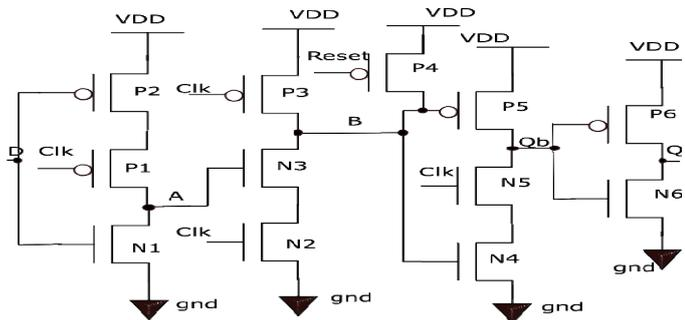
Fig. 1. Positive edge triggered TSPC DFF.
