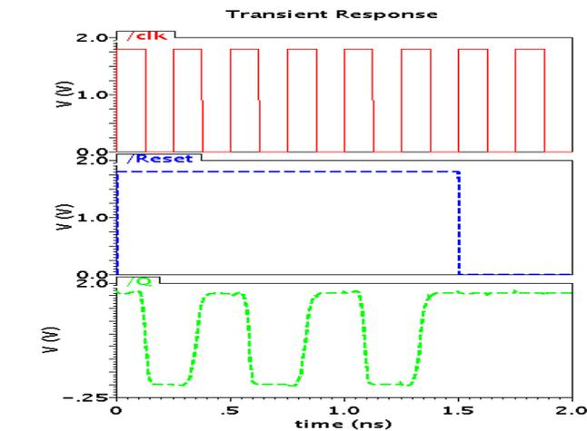
Fig. 6. Simulation results of toggle mode MTSPC DFF.
