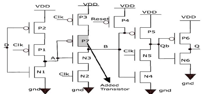
Fig.3. Positive edge triggered MTSPC DFF.
