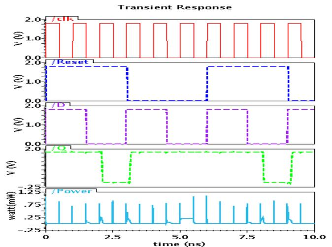
Fig.4. Simulation results of MTSPC DFF.
