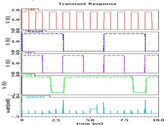
Fig. 2. Simulation results of TSPC DFF.
