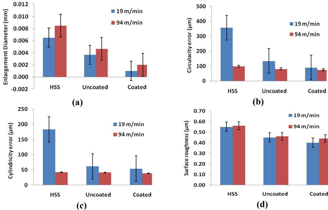
**Figure 2** Effect on the machining responses (a) enlargement diameter, (b) circularity error, (c) cylindricity error, and (d) surface roughness
