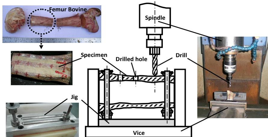
**Figure 1** Figures and schematics of experimental set-up
