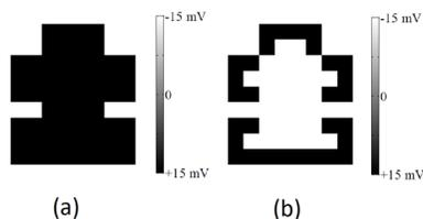
Fig. 9. Simulation results for the border extractor image processing function: (a) initial image and (b) final image.
