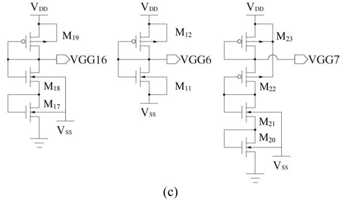
Fig. 2. Detailing of blocks in Fig.1: (a) Level shifter; (b) Current subtractor; (c) Voltage references.
