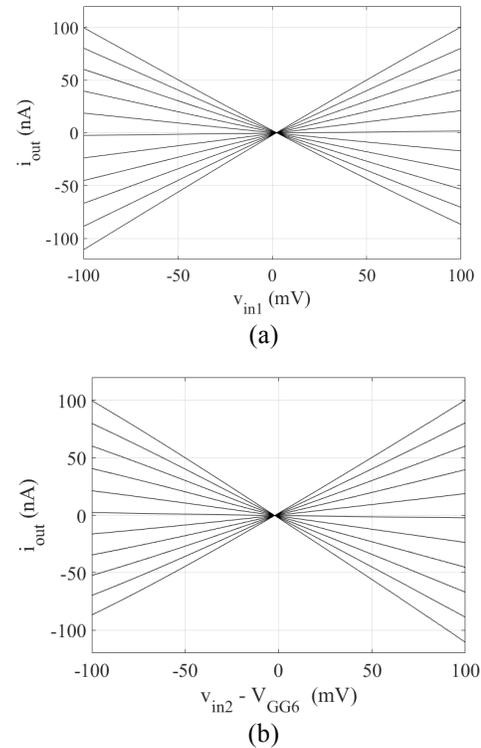
Fig. 3. Multiplier DC transfer characteristics: (a)  $i_{out}$  vs.  $v_{in1}$ , with  $v_{in2} - V_{GG6}$  varying from -100 mV to 100 mV with steps of 20 mV; (b)  $i_{out}$  vs.  $v_{in2} - V_{GG6}$ , with  $v_{in1}$  varying from -100 mV to 100 mV with steps of 20 mV. ( $V_{GG6} = 400$  mV).
