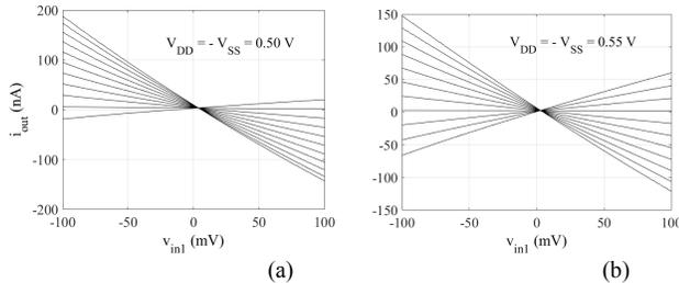
Fig. 6. Multiplier DC transfer characteristics  $i_{out}$  vs.  $v_{in1}$ , with  $v_{in2} - V_{GG6}$  varying from -100 mV to 100 mV with steps of 20 mV. Supply voltages  $V_{DD} = -V_{SS}$  equal to: (a) 0.50 V; (b) 0.55 V.
