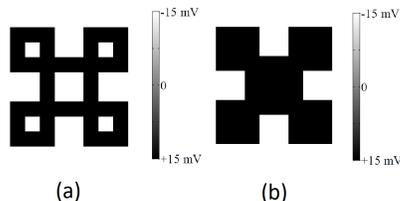
Fig. 8. Simulation results for the hole filler image processing function: (a) initial image and (b) final image.
