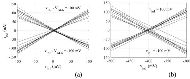
Fig. 5. Monte Carlo analysis for DC transfer characteristics: (a)  $i_{out}$  vs.  $v_{in1}$  with  $v_{in2} - V_{GG6} = \pm 100$  mV and (b)  $i_{out}$  vs.  $v_{in2}$  with  $v_{in1} = \pm 100$  mV.
