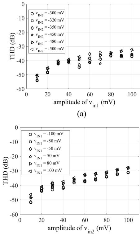
Fig. 4. Multiplier Total Harmonic Distortion: (a)  $v_{in1}$  sinusoidal (1 kHz) and constant  $v_{in2}$ ; (b)  $v_{in2} - V_{GG6}$  sinusoidal (1 kHz) and constant  $v_{in1}$ . ( $V_{GG6} = 400$  mV).
