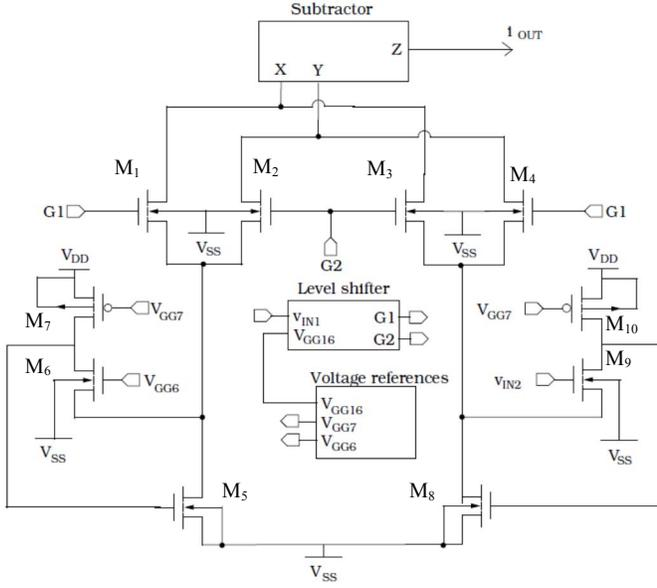
Fig. 1. Proposed CMOS analog multiplier architecture
