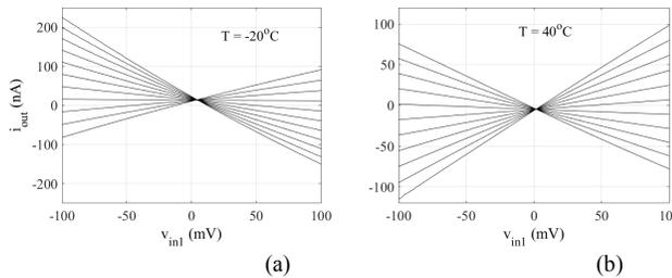
Fig. 7. Multiplier DC transfer characteristics  $i_{out}$  vs.  $v_{in1}$ , with  $v_{in2} - V_{GG6}$  varying from -100 mV to 100 mV with steps of 20 mV: (a)  $T = -20^\circ\text{C}$ ; (b)  $T = 40^\circ\text{C}$ .
