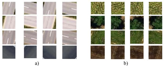
Fig. 4. Examples of boxes used for training (positive boxes, asphaltic road – Fig. 4.a and negative boxes – Fig. 4.b).
