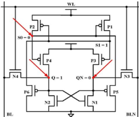
To write data 0 into the proposed 12T cell, word-line WL and bitline BL need to be 0 state, and bitline BLN must be 1 state. Subsequently, node Q will be pulled down to 0 state, and node QN will be pulled up to 1 state.
